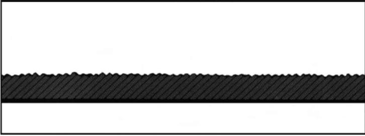
**1.** The surface of the substrate is blasted with an abrasive to roughen it, so other elements in the Excalibur process adhere to it better.
