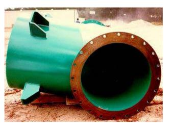
Scotchkote™ Fusion-Bonded Epoxy Coating 134 is a one part, heat curable epoxy coating that can be custom applied to protect pipelines (external and internal) and a variety of infrastructure components from corrosion.
