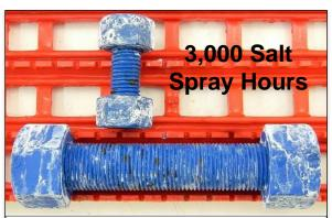
Photos Samples at 3,000 Salt Spray Hours conducted by Assured Testing Services. Coated by Southwestern Plating Company. Bolt Treatment: 0.3-0.5 mil zinc plating with 0.8-1.2 mil of 857G-018
